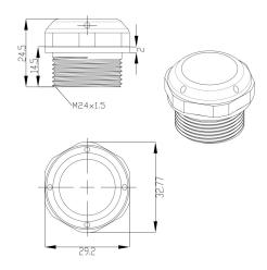
• Application wall thickness is up to 5.0mm when using the lock nut. B: Black color
